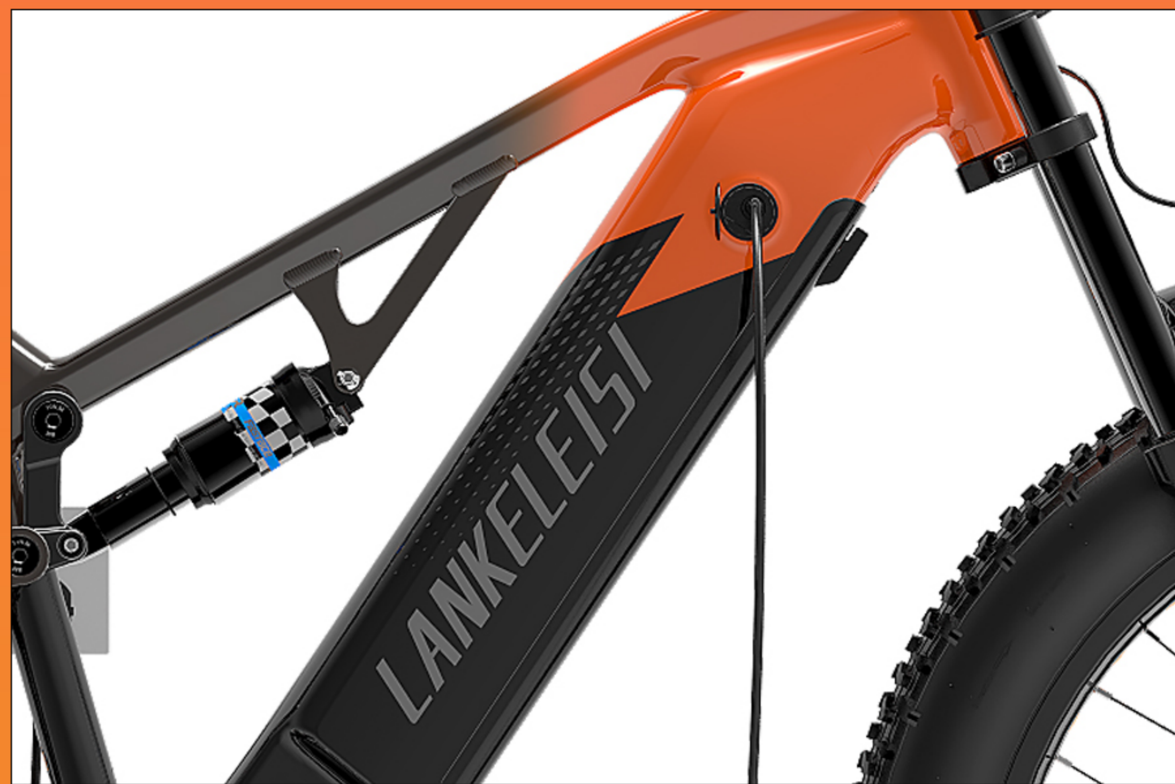
A. Recharge the battery on E-Bike directly
